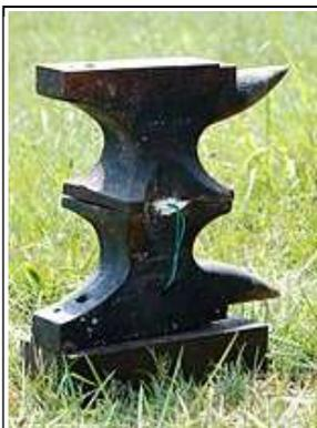
A prepared anvil. Gun powder is in a chamber between the anvils and visco fuse.
