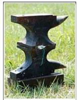
A prepared anvil. Gun powder is in a chamber between the anvils and visco fuse.
